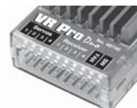
VR Pro Duo has two battery input wires on the opposite side. It can be connected with two batteries for power supply. VR Pro Duo can also connect 1 piece of battery for work.(We suggest to use Dualsky 20C series 2S li-po battery for VR Pro Duo) When these wires are connected correctly, please remove the FSS-3 plug pin to work.
